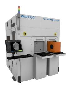
WX3000 systems are designed specifically for various wafer-level and advanced packaging applications including wafer bumps, solder balls and bumps, gold bumps and copper pillars. The systems provide superior measurement and inspection performance for features down to 25-micron, including bump height, coplanarity, diameter and shape, relative location and a variety of other measurements.
